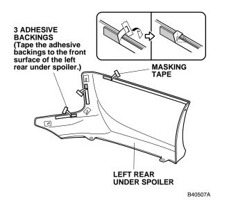
7. Using one alcohol swab, thoroughly clean the rear bumper where the left rear under spoiler will attach.
