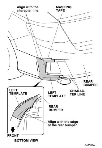
3. Using a pushpin, pierce the rear bumper through the four holes in left template. Remove the left template.
